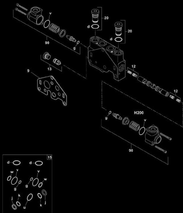
**CONTROL VALVE ASSY > VALVE ASSY, CONTROL > BOOM**
