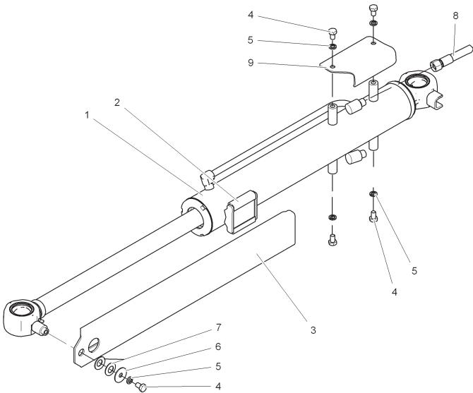
**VEHICLE > BOOM CYLINDER ASSY > BOOM CYLINDER,
