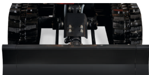
Extended undercarriage 840 mm - Increased stability
