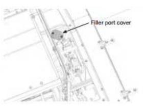
Interval for checking/greasing: 500 hours
