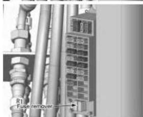
Check the fuse for wire blown.
