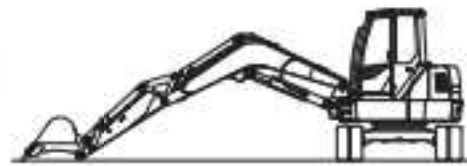
Posture of discharging hydraulic oil
