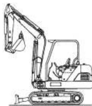
Bucket position at the time of sealing off hydraulic oil tank.
