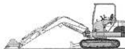
Bucket position at the time of checking the hydraulic oil level.
