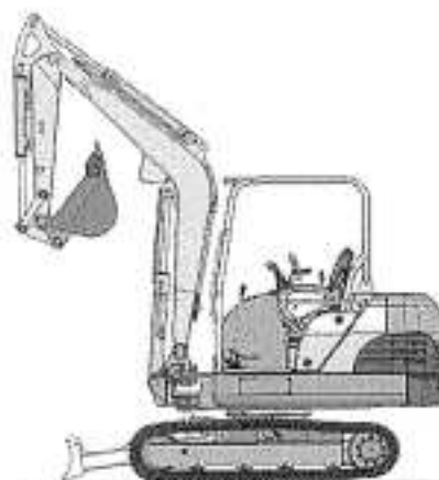
Bucket position at the time of sealing off hydraulic tank.
