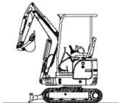
Bucket position at the time of sealing off hydraulic tank
