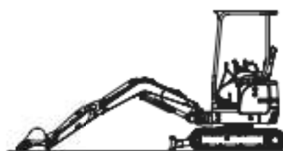
Bucket position at the time of checking the hydraulic oil level.
