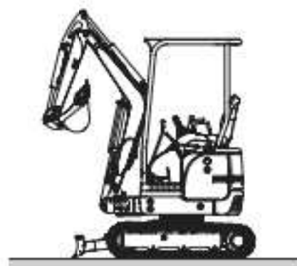
Bucket position at the time of sealing off hydraulic tank.
