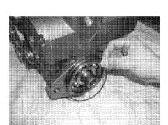
9. Remove shaft(U001) with bearing from housing.
