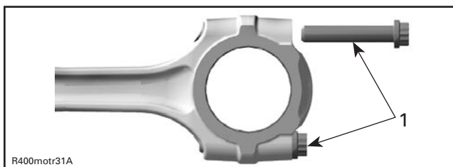
1. Connecting rod screw
